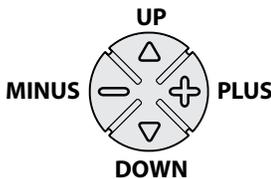
**Set the current time** using the PLUS and MINUS keys. By holding the key down the time will change rapidly. A tap will cause a stepped change. Once you have set the correct time, use the DOWN arrow key to move to the next section.
