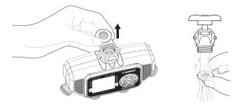
Activate the MANUAL mode by pressing the MANUAL button. Open all of the valves and spray water through each valve and the faucet connection to flush out any built-up sediments
